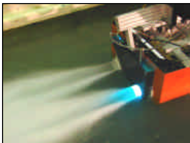
18-foot Waterjet-Propelled Model of the RV ATHENA Underway at DTMB
