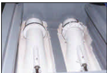
Waterjet Installation on the 18-foot RV ATHENA Model
