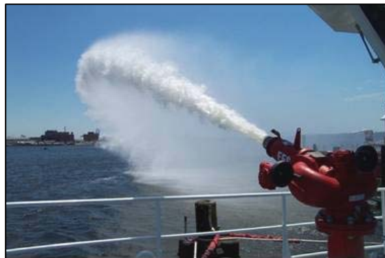
Unmodified Monitor – Note Breakup of Stream
