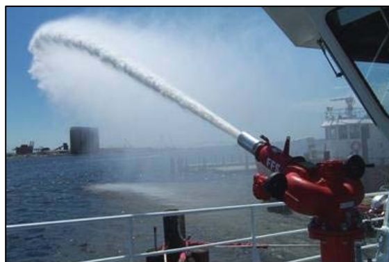
Existing Monitor with Vane Insert and Traditional Nozzle
