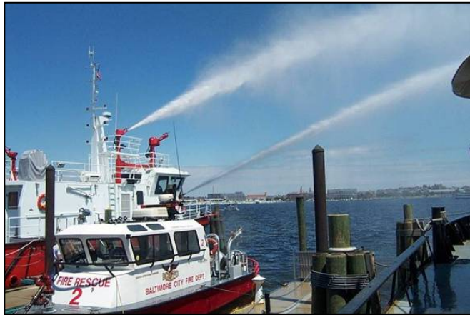
Comparison of Original, Unmodified Monitor (top) and the Final Design Solution (bottom)
